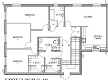
FIRST FLOOR PLAN G.E.A. 149.8 SQ M G.I.A. 134.4 SQ M N.T.A. NIL SQ M
